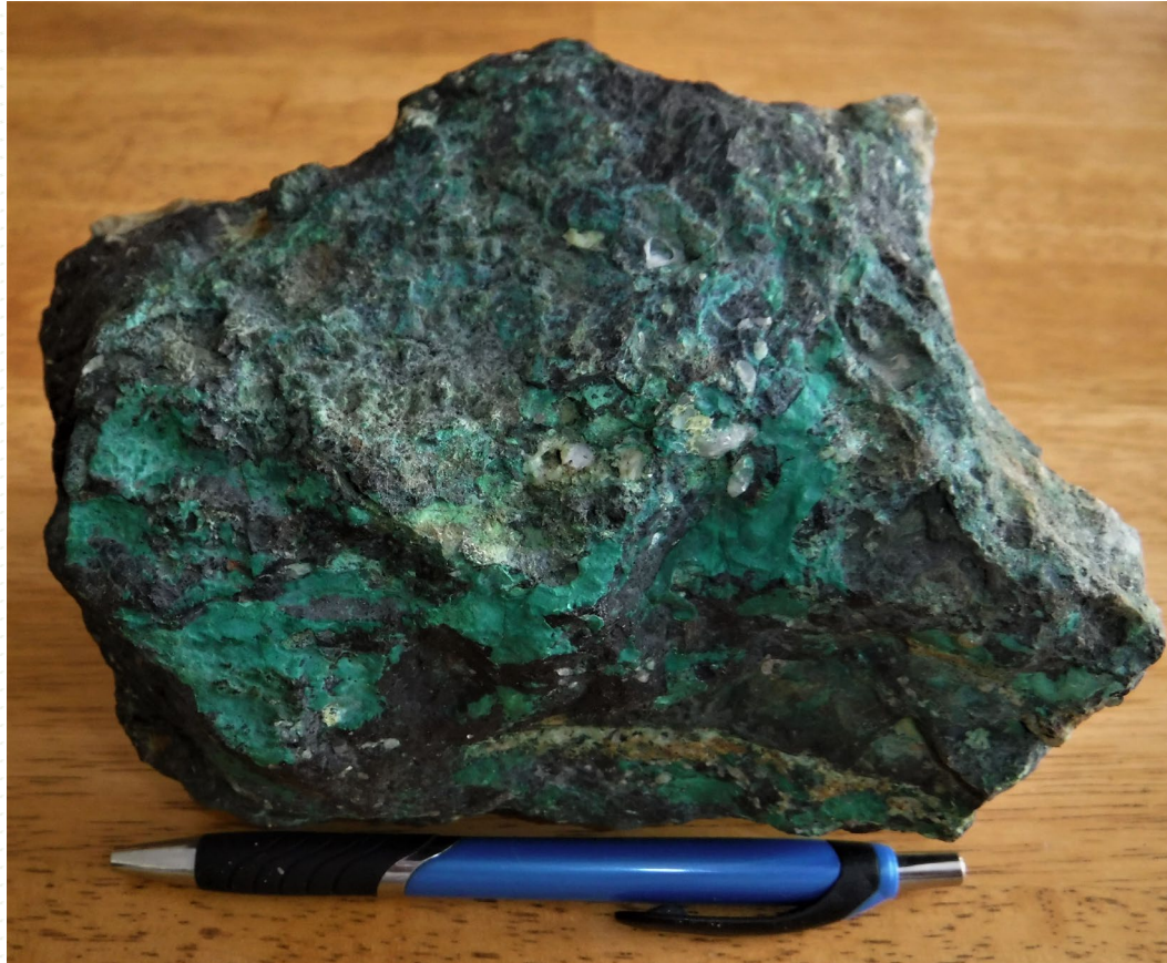
Massive chalcocite, 61.2% Cu, 5600gpt Ag south end of the property.
